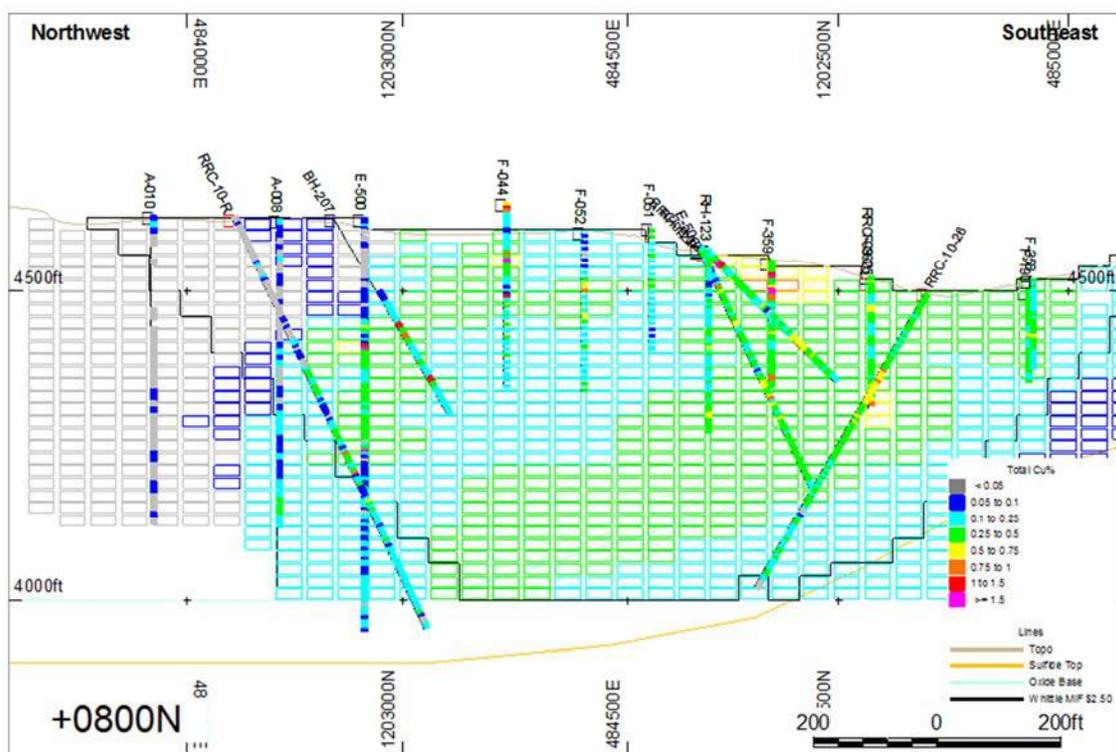
Figure 2: Cross Section Through Zonia Block Model (located at local grid northing +800N)
