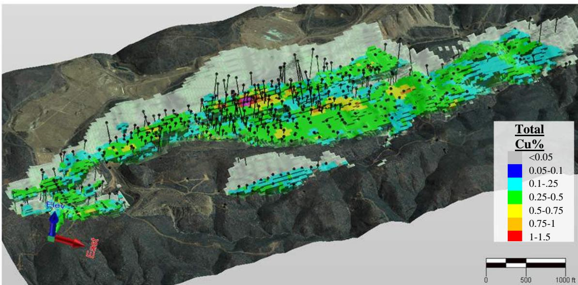
Figure 1: 3-D View of the Zonia Resource Blocks Looking Northwest (constrained at 0.2% cut-off).
