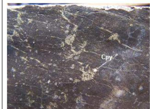
DDH-05-SF-09 – San Fernando: Pervasive potassic alteration (biotite – magnetite – K-spar) cross-cut by chalcopyrite veinlets and disseminations.
