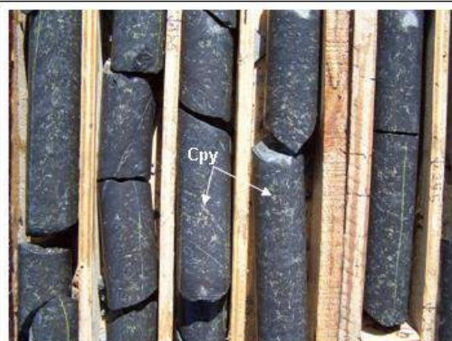
DDH-05-SF-05 - San Fernando: Pervasive potassic alteration (biotite – magnetite – K-spar) cross-cut by chalcopyrite veinlets.
