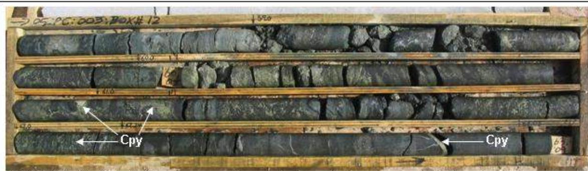
DDH-05-PC-03 - Picale: Massive magnetite – actinolite – chalcopyrite –(pyrite) mineralization.
